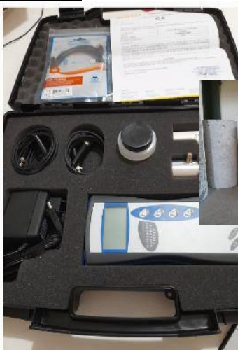
Velocity Primer (VP), Compression wave velocity (CWV)
